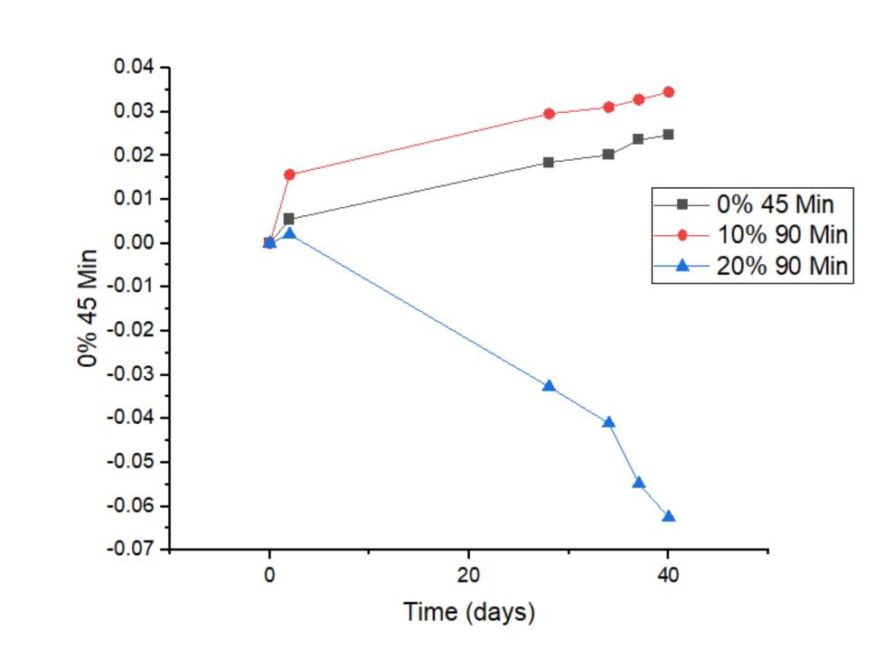
Swelling in Hysol epoxy was also investigated, and the data for this test is shown below. Hysol exhibited almost identical trends to the DP420 epoxy used for all other experiments, but 20% samples lost mass less than other samples. The effect of salt concentration is also shown here. Low salt and water samples are often very similar, but high salt samples seem to swell very differently. Each high salt sample swelled very slightly and similarly.
