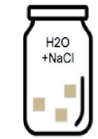
**Absorption**: HDP420 was mixed with concentrations of 0,10, 20, 30 wt.% toluene to create cubes of 1 cm<sup>3</sup> cured at 60°C for 35 minutes. Each of the cubes was soaked in individual vials containing solutions of either just DI water, low salt, or high salt concentrations.
