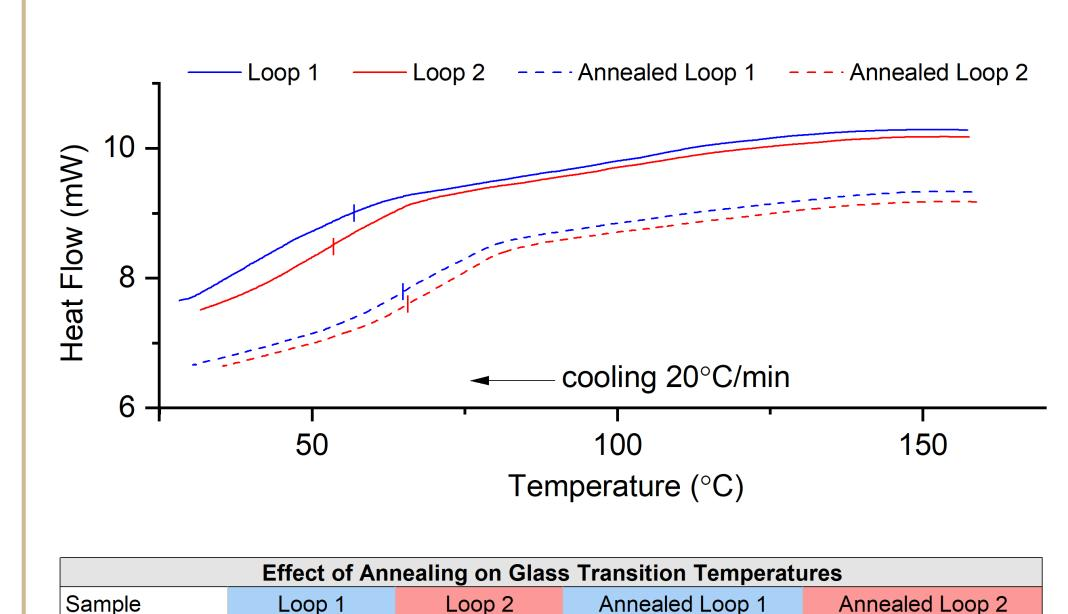
DSC data and resulting glass transition temperatures (Tg) are shown in the graph and table above. The unannealed samples showed a larger difference in Tg of approximately 3°C. The annealed sample maintained a more consistent Tg and showed an overall similar behavior between loops compared to the unannealed sample.
